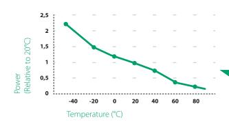
PTC (Positive Temperature Control) refers to the characteristic of the unique PTC paste used to generate the heat in the ROTAID – PTC AED cabinet heater. The resistance in the heat generating paste will increase with temperature to such an extent that it is limiting the power efficiently above 30 °C. This means that the heater will give more power when needed at low temperatures and less power as the temperature increases.
