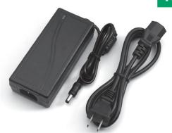
DC24V - 5000mA Power supply AC 100 ~240V 50/60Hz Input Cable length 1.2 mtr. Output DC 24 V± 5% Max. output current 5000mA - 120W. Connection **DC** -straight connector Cable length 1.8 mtr.
